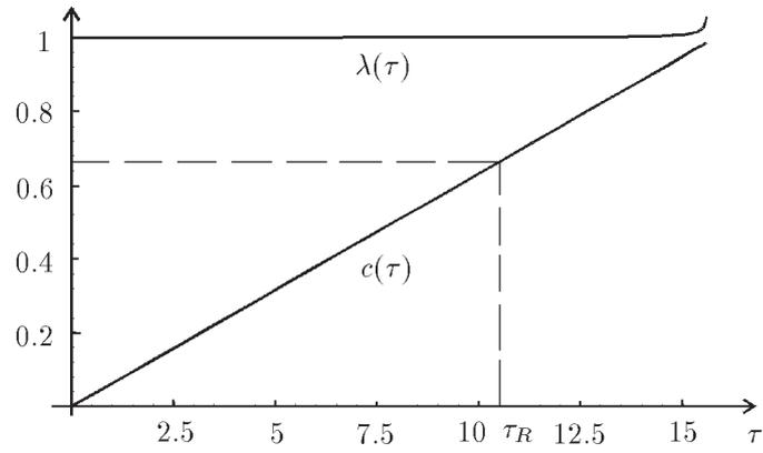
Fig. 1. Longitudinal extension  $\lambda = l/l_0$  and damage  $c$  as functions of dimensionless time  $\tau = t/t_*$ ; initial strain  $\varepsilon_0 = 0.0001$  corresponding to “brittle” rupture.
